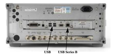
In addition, the Agilent IO Libraries CD that was included with your instrument contains USB Host drivers that allow control of other instruments connected to the USB bus.
